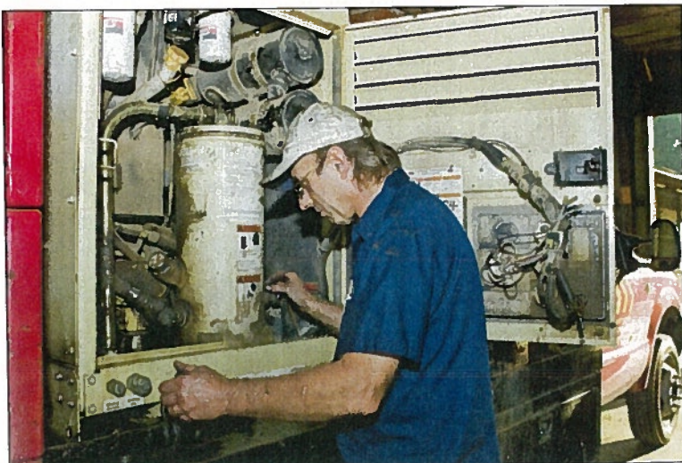
Kenny Belsar, mechanic, repairs an air compressor.
